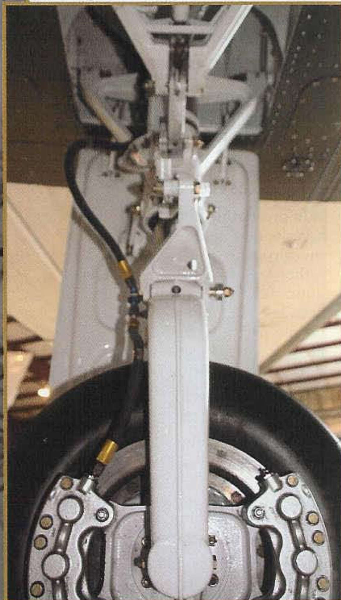
The overhauled landing gear is stripped and inspected for condition, and then all new hardware is used.
