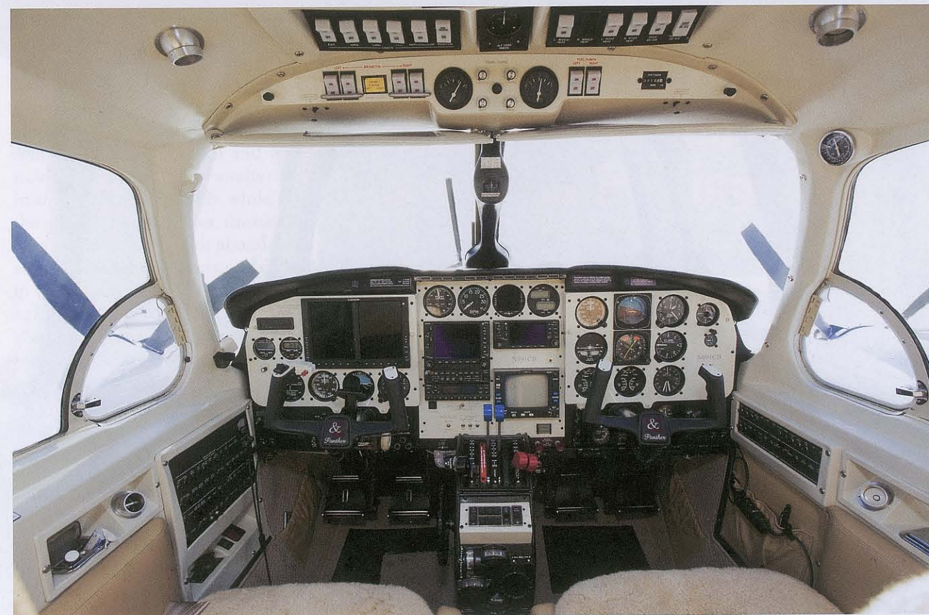
The Garmin G600 with synthetic vision provides a completely modernized cockpit. The Lock & Key renovation adds leather-covered control wheels, new internally lit overhead rocker switches, and panels with lettering etched into the surface.
