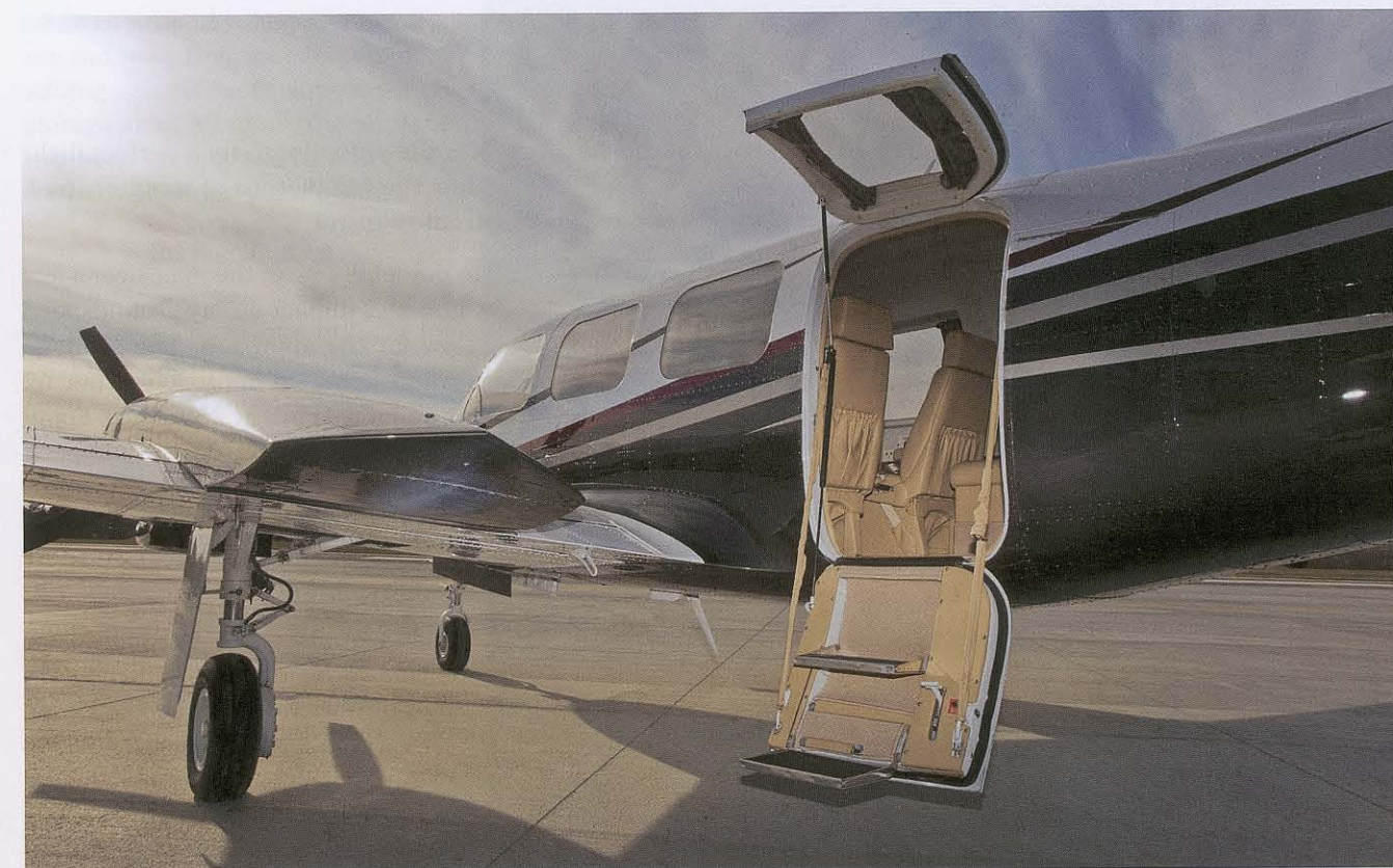
Entering the Navajo is an easy task thanks to large clamshell airstair door. Ample storage space is available in the aft cabin, wing lockers and forward nose compartment.
