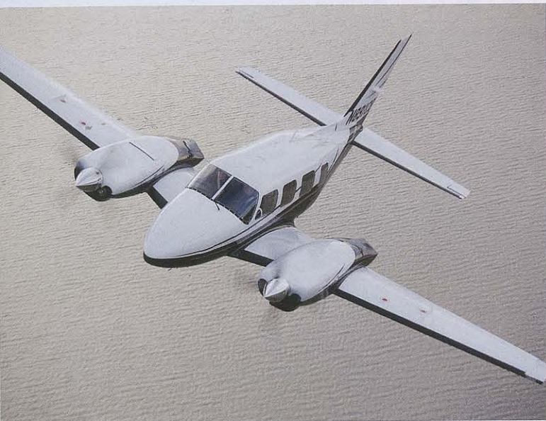
The Navajo is fitted with the Colemill Panther Lycoming TIO-540-J2B 350-hp turbocharged engines and also sports American Aviation aftermarket intercoolers. Hartzell four-blade, 74-inch diameter Q-tip propellers make for a quieter ride.
