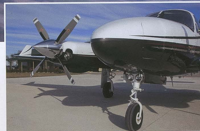
The Navajo is easy to manage in the pattern with up to 40 degrees of flaps available. HID landing lights provide 1 million candle-watt power and draw only 5 amps.
