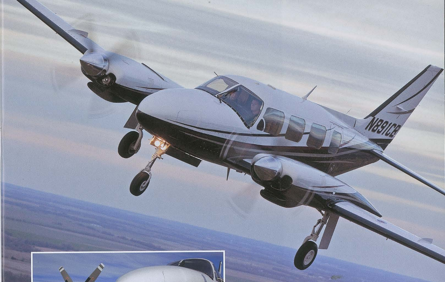
The Navajo is easy to manage in the pattern with up to 40 degrees of flaps available. HID landing lights provide 1 million candle-watt power and draw only 5 amps.
