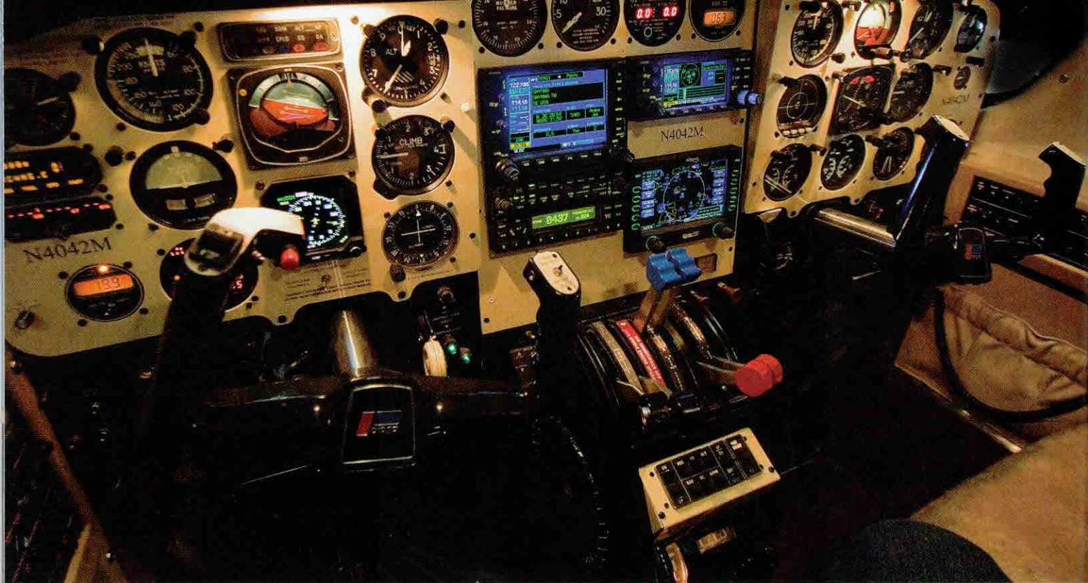
The Panther comes with a new Garmin nav package, a King Digital EFIS, an Avidyne MFD, TCAS and Stormscope. Every detail, inside and out, is transformed into cabin-class elegance.
