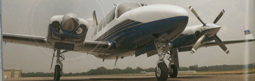
A "Lock and Key" Navajo gets a Colemill Panther conversion as part of the deal. This includes new or overhauled engines, plus new Q-tip propellers, prop governors, engine mounts, winglets, and more.
