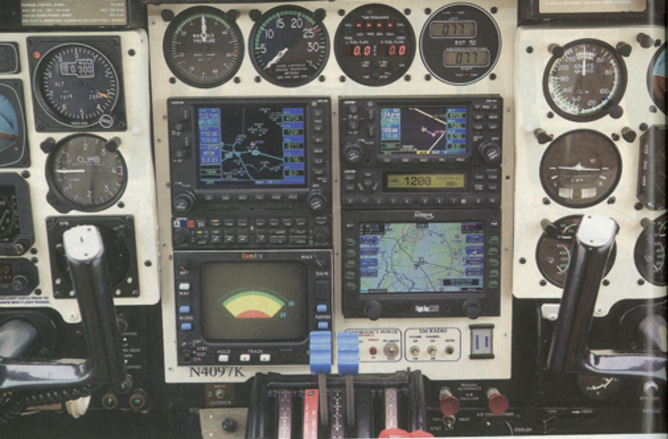
The instrument panel fast-forwards to the 21st century, with Garmin GNS 530/430 GPS/navcoms, an Avidyne FlightMax EX500 multifunction display, XM datalink weather, and your choice of either a Bendix/King KFC 200 or an S-Tec System 65 autopilot/flight director.
